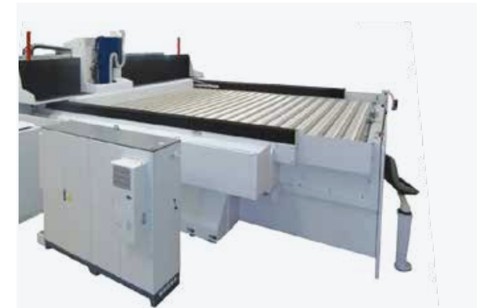
Bellows-type roof for dust and aluminium chips control
