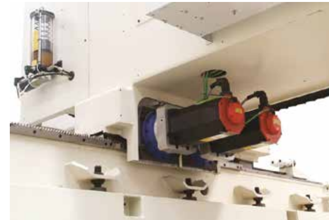
Kinematics with two drive motors on linear axes: backlash recovery, higher rigidity
