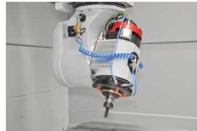
5 axes milling unit with direct drive technology
