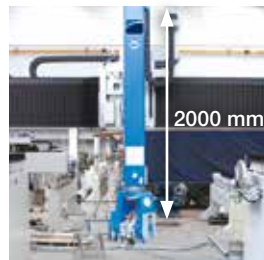
Z axis stroke up to 2000 mm
