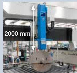
Z axis stroke up to 2000 mm
