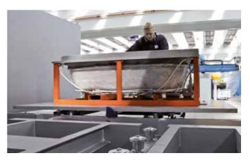
Mould carts with a mould lifting system
