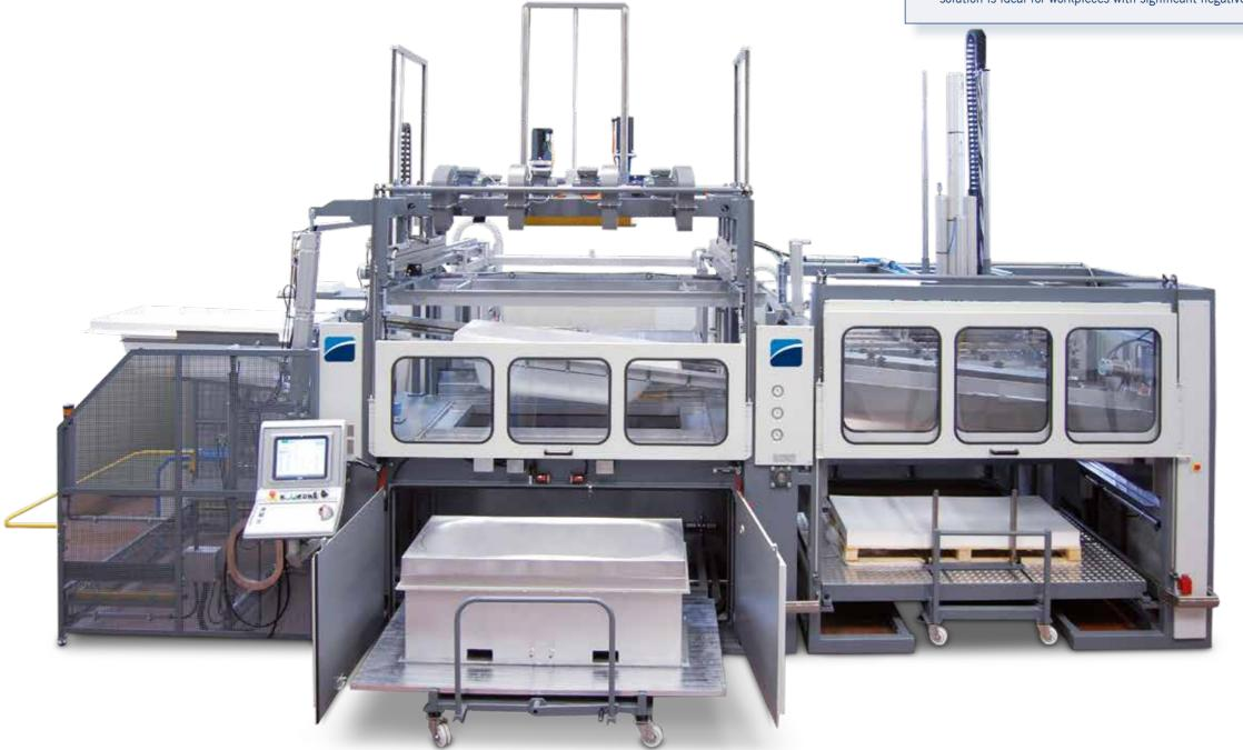
+ Intelligent heating management with thermal vision and advanced management using the exclusive CMS ThermoProphet function (patented). A thermal imaging camera allows point-to-point detection of the thermal impression of the sheet and automatically modifies the working percentages to guarantee the highest quality even in the presence of environmental variables. 55% lower
