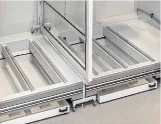
Conveyor belt under the table for chip removal
