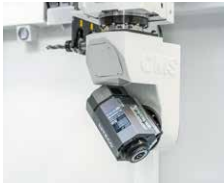
CX5 working unit Rigid and compact, with spindles from 8 kW up to 10 kW in 24,000 and 40,000 rpm versions for machining workpieces continuously with 5 axes.
