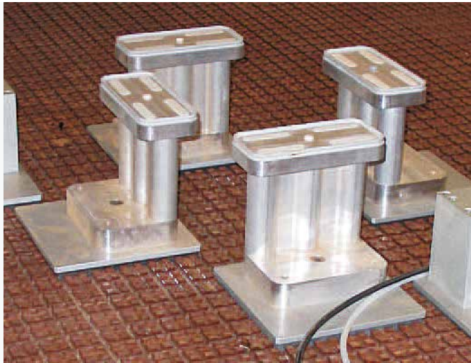
Suction and reference blocks for maximum flexibility in locking the piece
