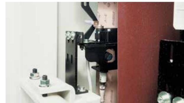
**PHOTOCÉLULES AVEC SYSTÈME DE "SUPPRESSION DE L'ARRIÈRE-PLAN" POUR GARANTIR À TOUT MOMENT LE CENTRAGE CORRECT DE LA BANDE ABRASIVE**
