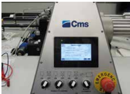
Software-based electronic control of cutting pressure
