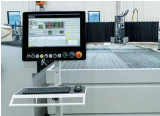
21,5" touch screen control panel on mobile trolley.
