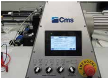
Software-based electronic control of cutting pressure
