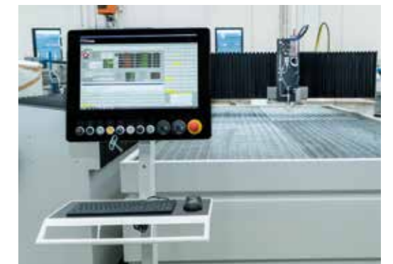
21,5" touch screen control panel on mobile trolley.
