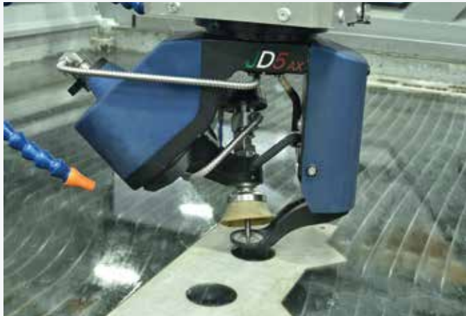
5-axis cutting head with JDC technology - Jet Drive Compensation -. ffective head management to carry out inclined cuts and check cut conicity (Opt)
