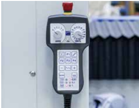
Remote pushbutton pad to control up to 6 axes that allow you to operate close to the cutting surface and set multi-origins (optional)
