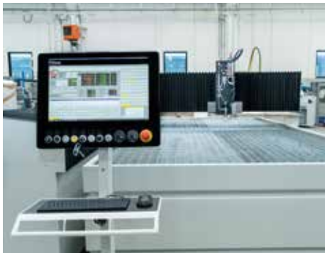
Console on a mobile trolley with 21.5" touch screen (optional)
