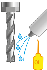
Air blower with micro-lubrication Blower with air and a small amount of oil suitable for lubricating and cooling the tool when machining non-ferrous metals.
