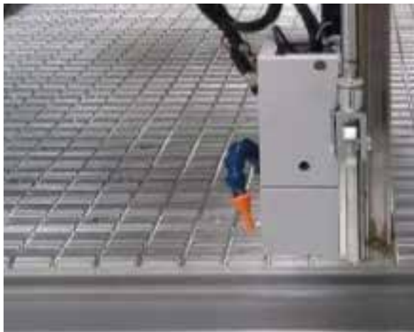
OPTISCOUT Device for measuring reference points on plastic or paper material, for rotranslation of the program according to the actual workpiece position on the bed.
