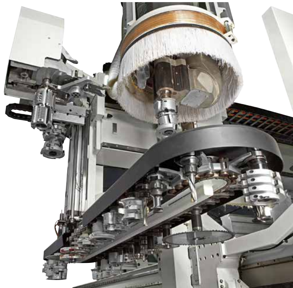
MACH 5 This device performs a tool change in just five seconds, drastically reducing downtime time.
