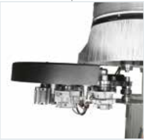
Circular 12-position magazine located on the operating unit.
