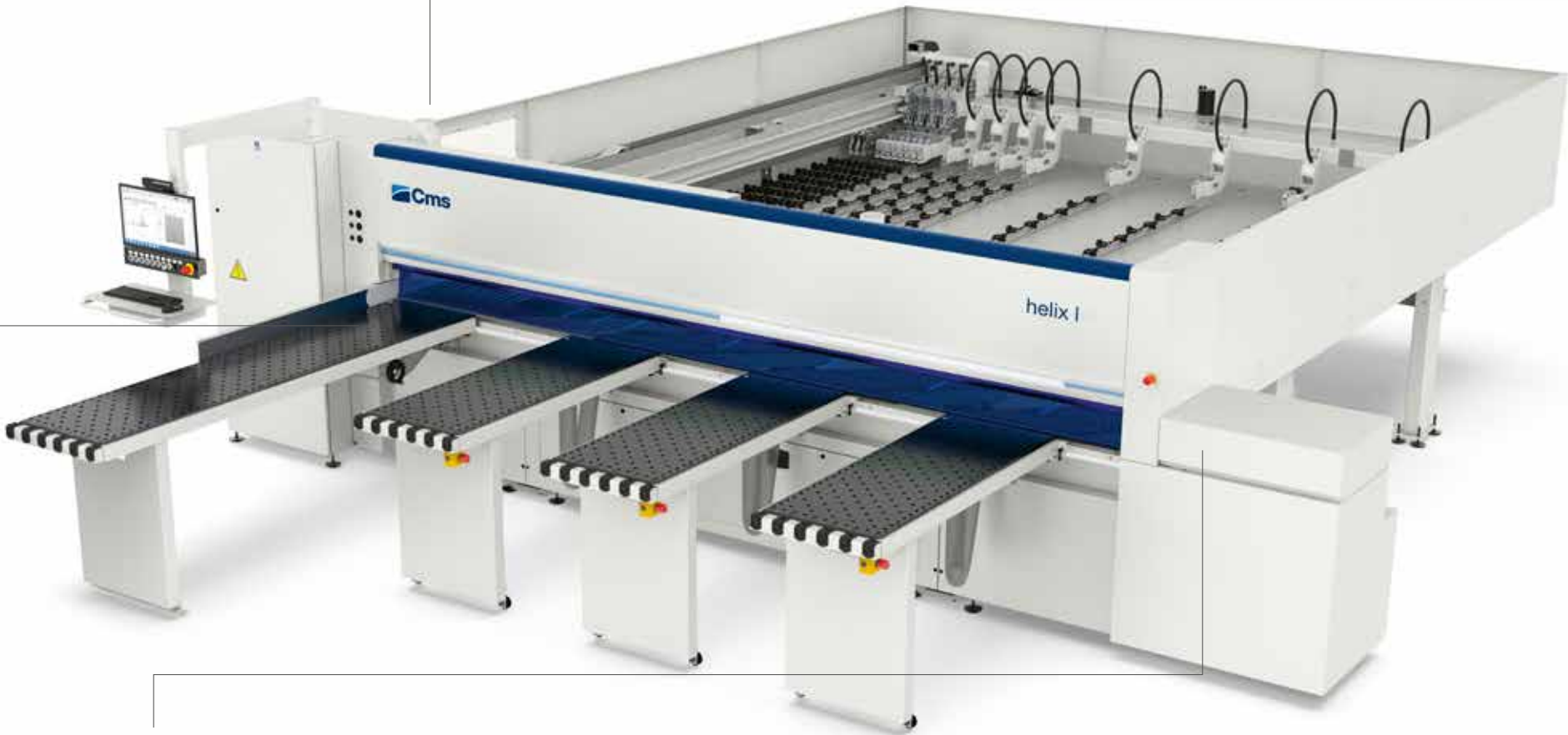
New blade carriage for easy inspection and maintenance. With maximum power up to 18 kW.
