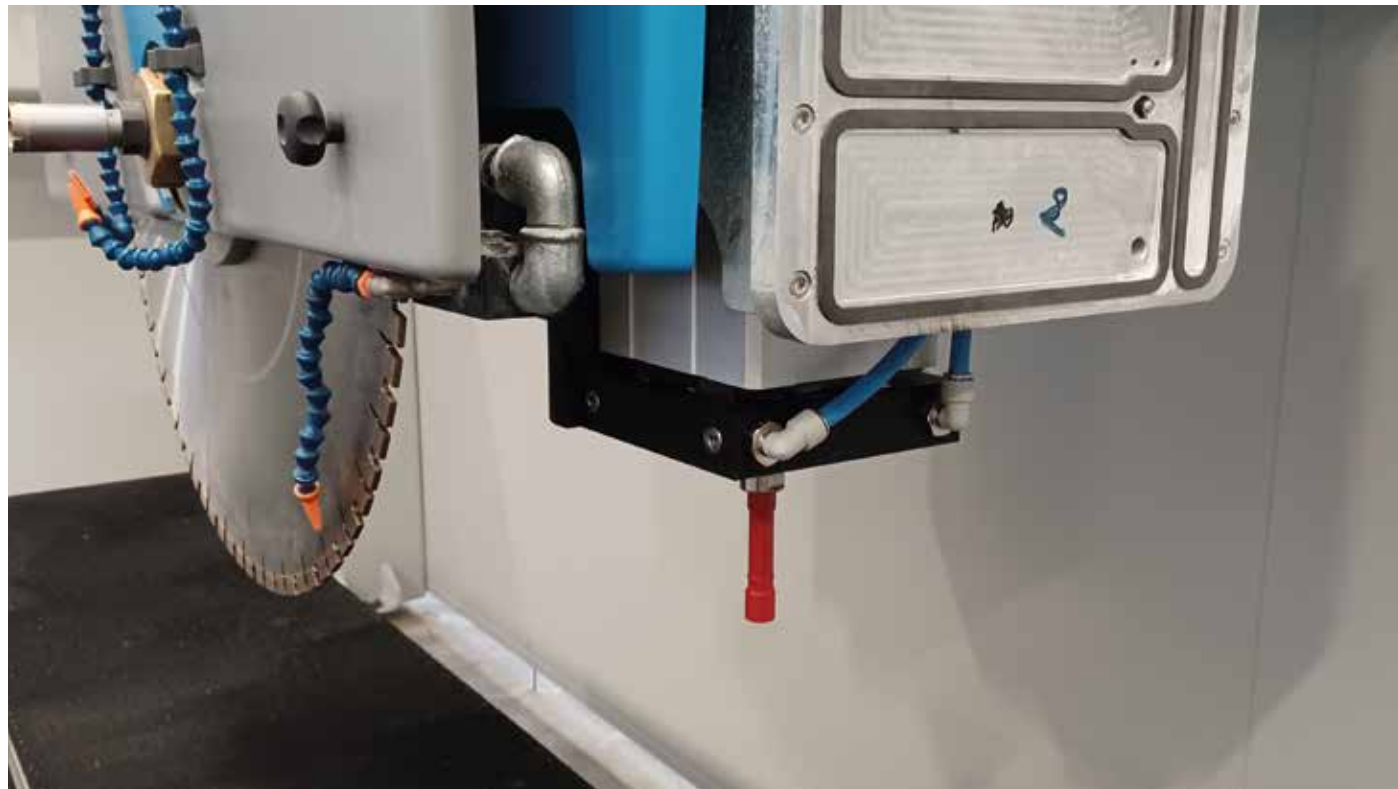
SIDE SPINDLE: additional 3.7 kW 14,000 rpm side spindle with manual tool change. It allows an additional tool to perform milling, drilling, lettering, engraving and bas-reliefs without having to remove the tool from the main motor. It can be used for high-speed machining that cannot be handled with the blade motor alone.
