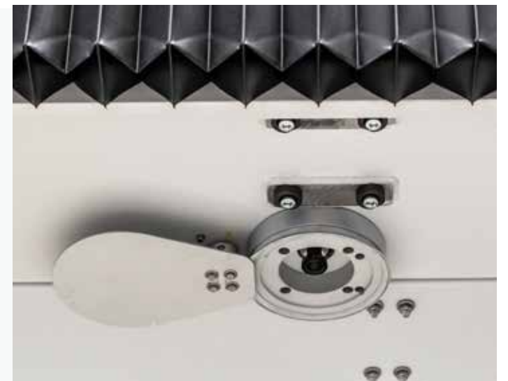
CAMERA: system to obtain the images from the working table, it permits to accellerate the pieces positioning and notice possible bugs on the slab
