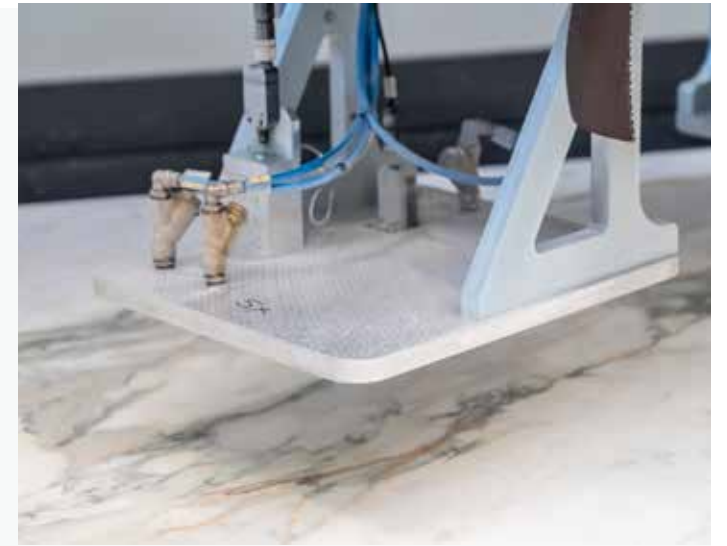
SLAB THICKNESS PROBE for the automatic measuring of the piece thickness
